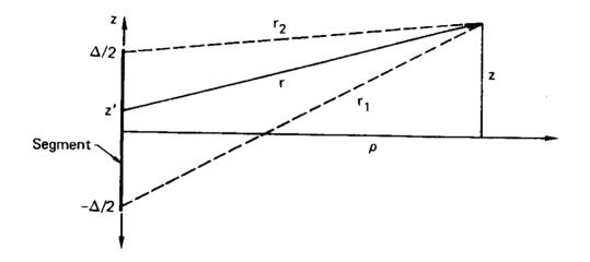
Figure 7. Coordinates for Evaluating H Field of a Segment.
