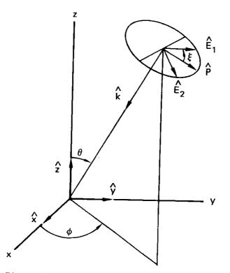
Figure 4. Coordinate Parameters for the Incident Plane Wave.
