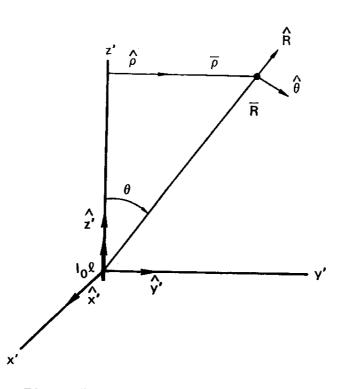
Figure 5. Coordinate Parameters for Current Element.
