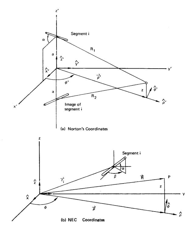
Figure 6. Coordinate Systems Used to Evaluate Norton's Expressions for the Ground Wave Fields in the NEC Program.
